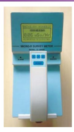
Micro R Survey Meter (Digital) Model D-MRSM is a portable, Si-Lab micro-controller based, battery operated instrument for measurement of environmental low level gamma radiation dose rate. It employs an internally housed 1"x1" NaI(TI) detector integrally coupled to a 1" dia PMT offering optimum performance to lower energies.
