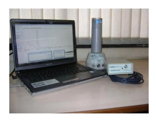
GSpec ADC is a versatile compact USB based 1024 channel Multi Channel Analyzer GSpec-ADC is powered by USB interface It contains 1024 channel 48 MHz Wilkinson ADC with Silab Microcontroller for USB interface with PC for spectrum acquisition and data processing.
