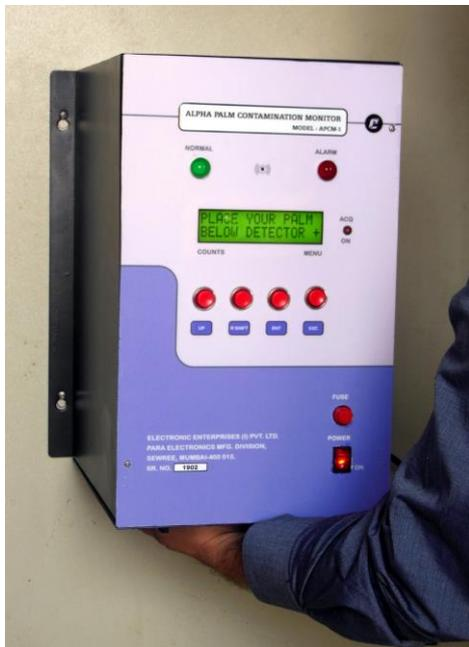
Model APCM-1 is a wall mountable Alpha Palm Contamination Monitor developed for measurement and detection of alpha contamination on Palm. APCM-1 is designed and manufactured indigenously by Para Electronics Mfg. Division of Electronic Enterprises (I) Pvt. Ltd., Mumbai, India.
